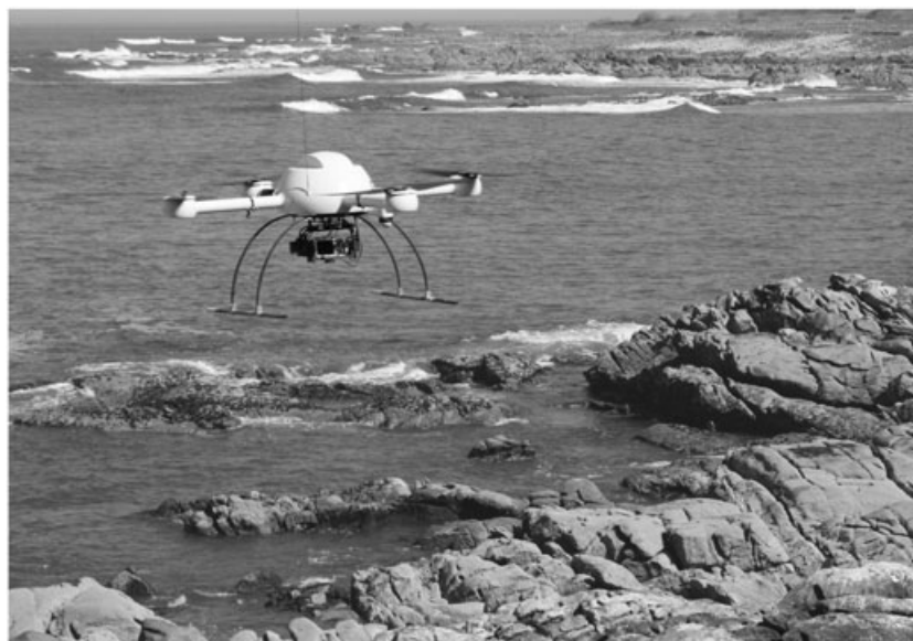
Figure 5. The md4-200 micro-drone flying over Oia on 24 April 2013. The camera is slung beneath the vehicle. The micro-drone measures 0.54 m from rotor shaft to rotor shaft, has a mass of about 0.8 kg and a maximum payload of 0.3 kg.
